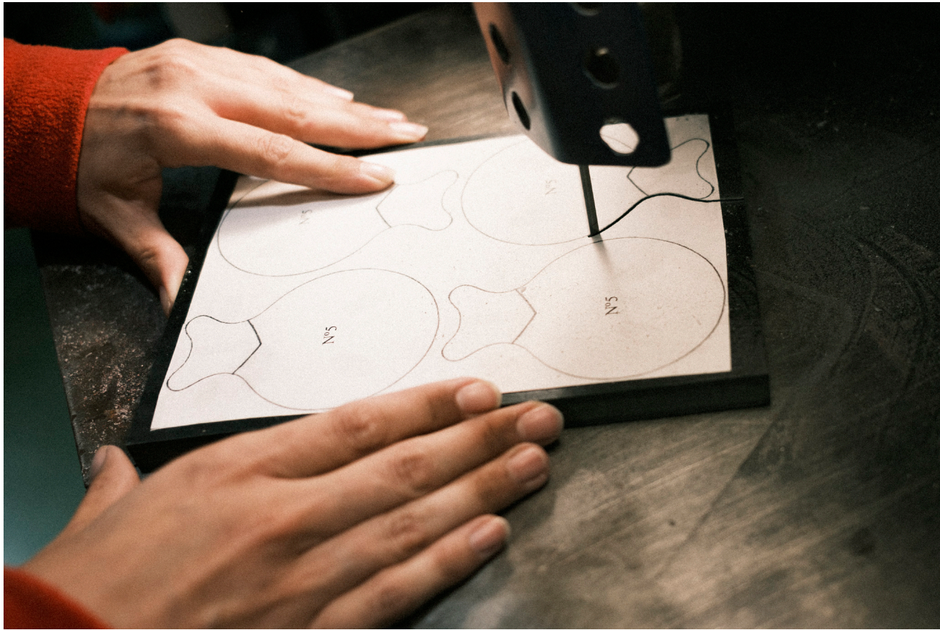
Cutting of a castanet in the Castañuelas del Sur workshop (Sevilla)
